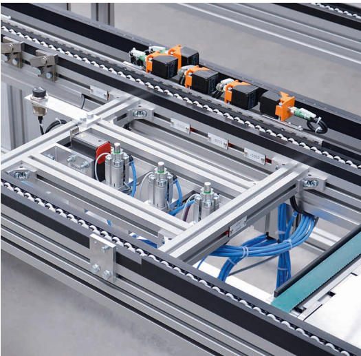
Versamove plus: Customer-specific special stopper unit with four removal positions
